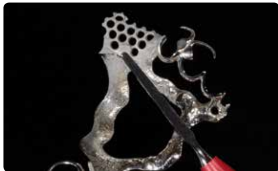
Carefully blast the retentions with \text{Al}_2\text{O}_3 (80–100 \mu\text{m} ) at 3 bar (44 psi) pressure; then remove any residue by careful tapping with an instrument.
