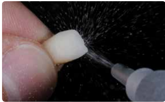
Create the cut-back. Sandblast the surface with \text{Al}_2\text{O}_3 (80–100 \mu\text{m} ) at 2 bar (29 psi) pressure.
