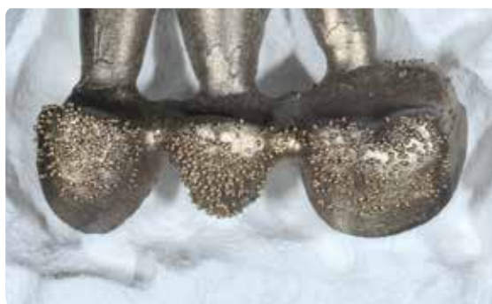
Carefully divest, blast and pickle the framework on the model.
