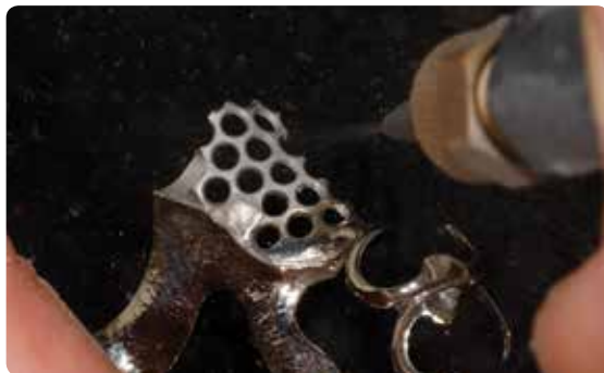
Carefully blast the retentions with \text{Al}_2\text{O}_3 (80–100 \mu\text{m} ) at 3 bar (44 psi) pressure; then remove any residue by careful tapping with an instrument.
