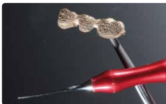
Carefully blast the framework with \text{Al}_2\text{O}_3 (80–100 \mu\text{m} ) and 2–3 bar (29–44 psi) pressure and tap off with an instrument.
