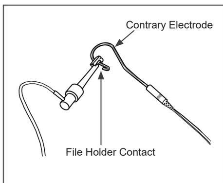
2. Check that the probe cord is properly plugged into the jack.
