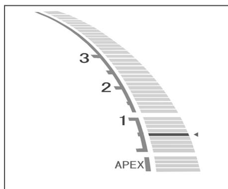
5. Touch the contrary electrode with the file holder's contact tip. Check that all the canal length indicator bar on the display are lit, the word "APEX" flashes and audible beep becomes continuous.
