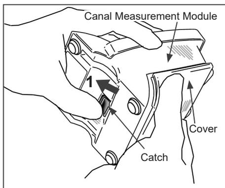
1. Hold the cover and slide the catch on the bottom of the module towards the display to release it.
