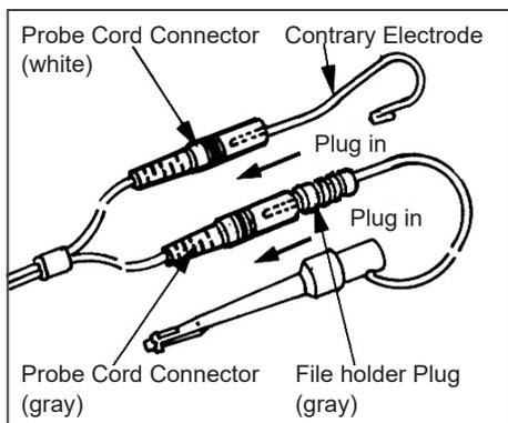
2. Insert the file holder's gray male plug into the gray female connector on the probe cord. Insert the contrary electrode into the white female connector on the probe cord.
