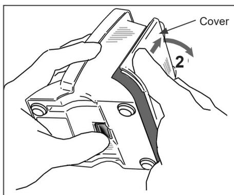
2. Slide the cover in the direction indicated by the arrow in the diagram to take it off.
