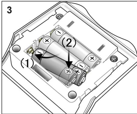
3. Take out the old batteries and replace them with new ones. Make sure the plus and minus poles are correctly lined up.
