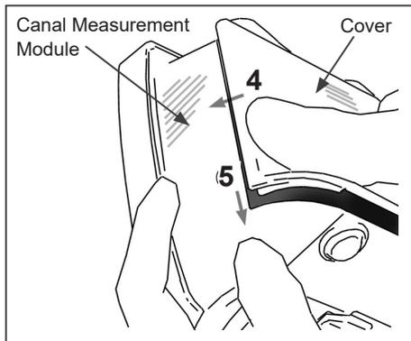
4. Line up the projections on the cover with the notches in the module. Fit the cover onto the module and slide it down into place.
