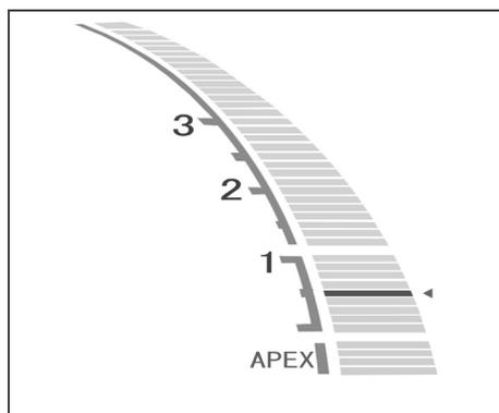
5. Check that all the meter indicator bars on the display are lit, the word "APEX" flashes and audible beep becomes continuous.
